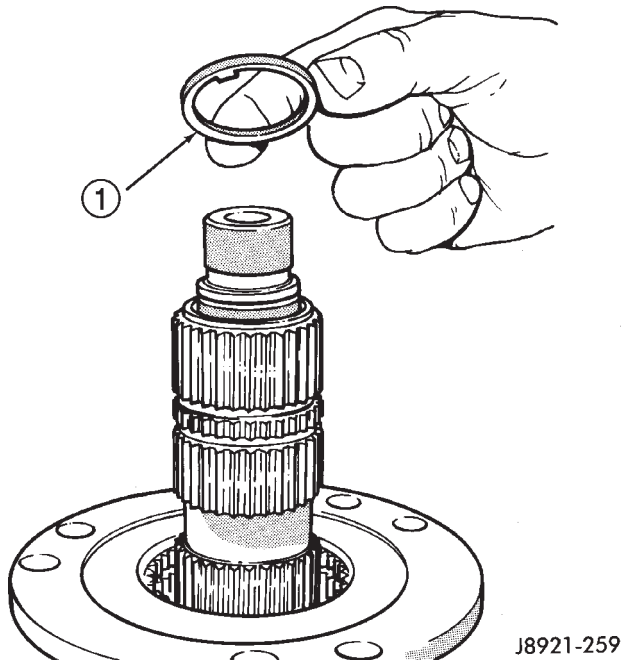
Fig. 75 Installing Clutch Shaft Thrust Washer
