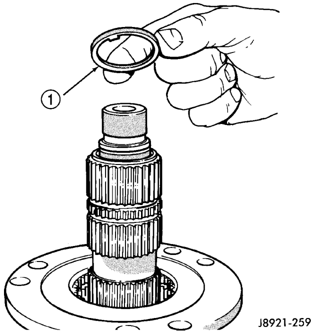
Fig. 28 Clutch Shaft Thrust Ring Removal
